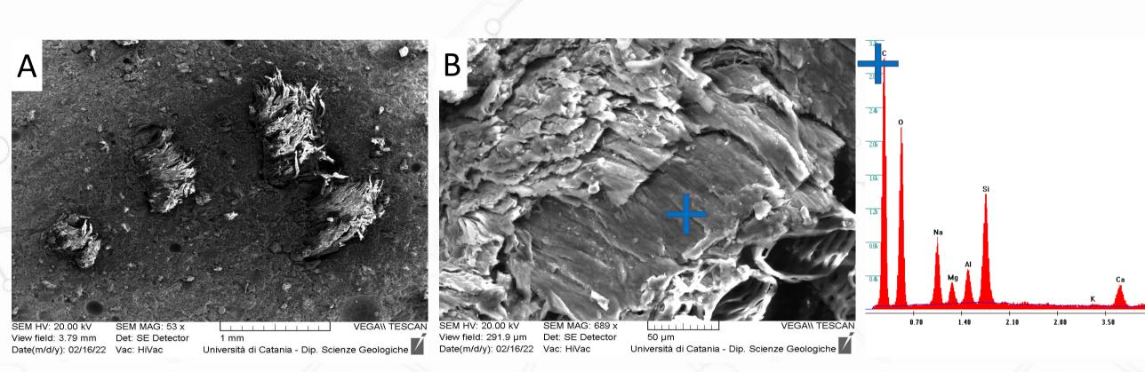
SEM images of samples made with prickly pear fibres (A-B). Image A shows the fibres perfectly enwrapped by the matrix. Image B shows the geopolymeric matrix on the top and the fibre on the bottom of the picture.
