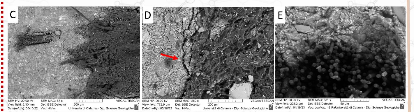
SEM-EDS images of samples made with palm tree (C-D) and carbon fibres (E). Image C shows a transition zone between palm tree fibres and the geopolymeric matrix. At that magnification the fibres seem to have an acceptable adhesion to the matrix. Image E, which is a magnification of image D, reports the existence of a fracture located in the geopolymeric matrix. The nature of these fractures is still under study. Image E shows a detail of the carbon fibres and the geopolymeric matrix.
