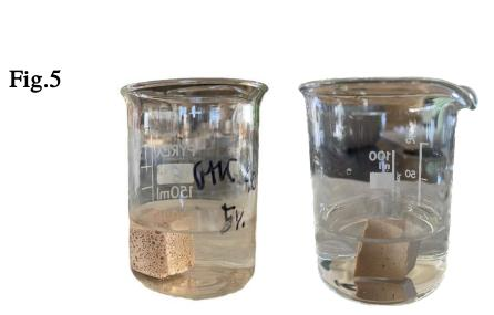
A test of integrity in water (Fig.5) was performed on MKgeopolymer samples, including the porous one, which showed undamaged surfaces after five days of immersion in distilled water.
