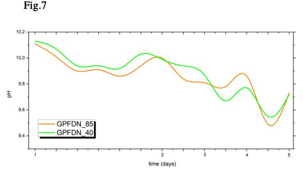
The figure (Fig.7) shows the pH variation of water containing sludge-based geopolymers (GPFDN\_85 and GPFDN\_40). Leaching leads the water pH to values slightly below 10 after 5 days, observing a marginally lower pH for the sample cured at 85°C for 5 hours.
