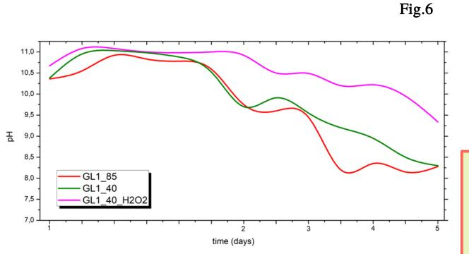
The figure (Fig.6) shows the pH variation of water after immersion of MK-based geopolymers GL1\_85 and GL1\_40 and the porous sample (GL1\_40\_H2O2) for a control time of 5 days. As evidenced, leaching leads to different pH values: the water in which was immersed porous geopolymer achieves pH above 9 after 5 days, whereas for the other samples pH decrease until 8.
