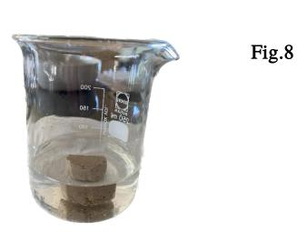
A test of integrity in water (Fig.8) was performed on FDN-based geopolymers, showing undamaged surfaces after five days of immersion in distilled water.
