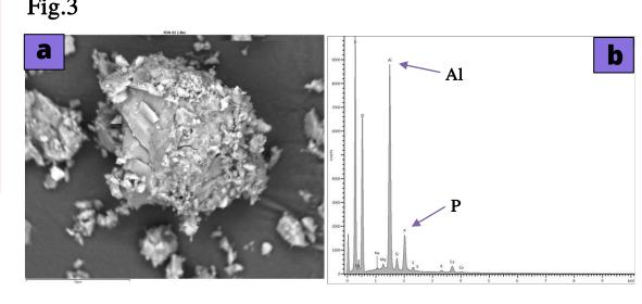
Chemical-morphological analyses by SEM-EDS (Fig.3) of magnified single granule of wastewater sludge (a) and correspondent EDS spectrum (b), showing aluminium and phosphorus as the main chemical components.
