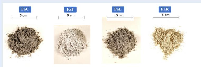
• Fly ashes recovered from the chimney filter of an industrial system.
