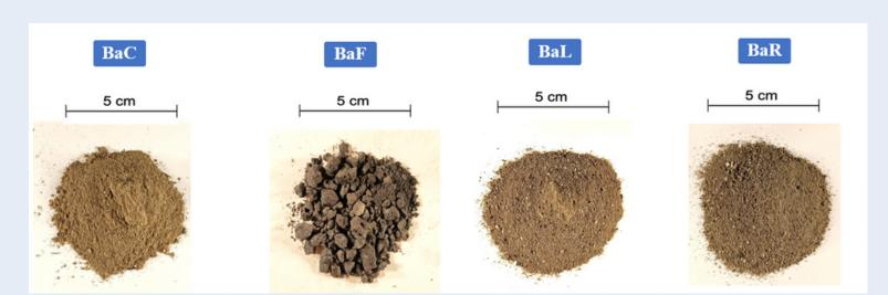
· Bottom ashes that accumulates inside the burner of the combustion chamber composed of slag and unburnt materials.
